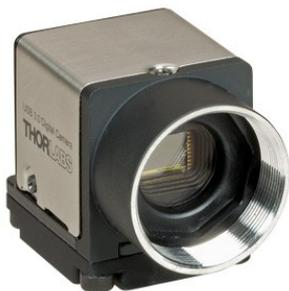
Compact, fast and lightweight. The new **DCC3240x**. The 29 x 29 x 29 mm small camera housing is not only ultra-compact, but due to its magnesium casing and a total camera weight of 43 g, it is also ultra-lightweight and robust. The powerful camera offers a bandwidth of 400 MByte/s via USB 3.0. Power is supplied via the USB bus, hence an extra power cable is obsolete.
